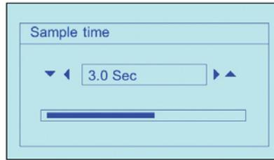
Use the ▲▼ buttons for coarse adjustment and the ◀▶ buttons for fine adjustment. A typical setting would be 3 seconds.
