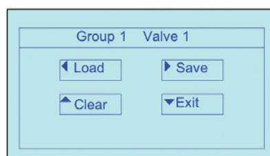
Using the **SAVE** command will overwrite the location with the current valve data.
